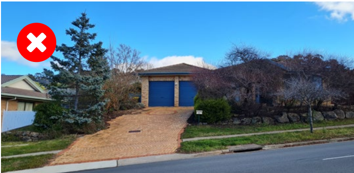
Undesired garage prominence to the street, with main dwelling and entrance fully screened
